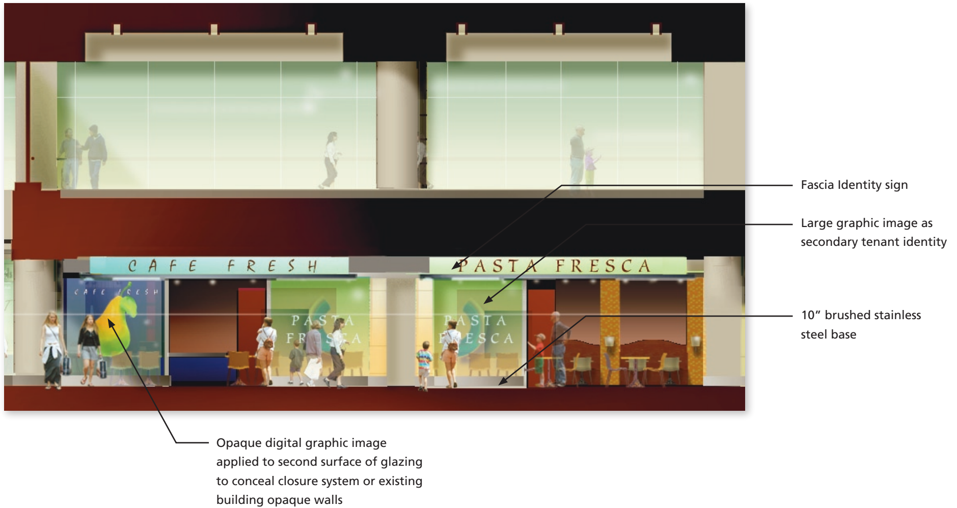
Tenant Space in Low Ceiling Common Area Condition
